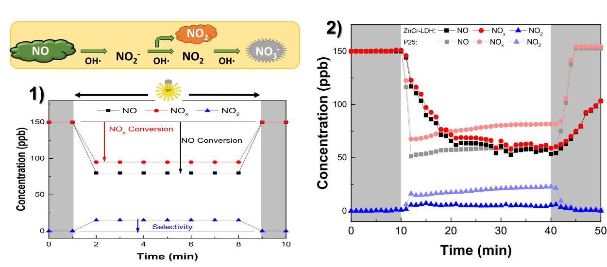
1) Example of photocatalytic test. 2) Photocatalytic test comparison of ZnCr-LDH (bold) and P25 (shadow) in powder.
