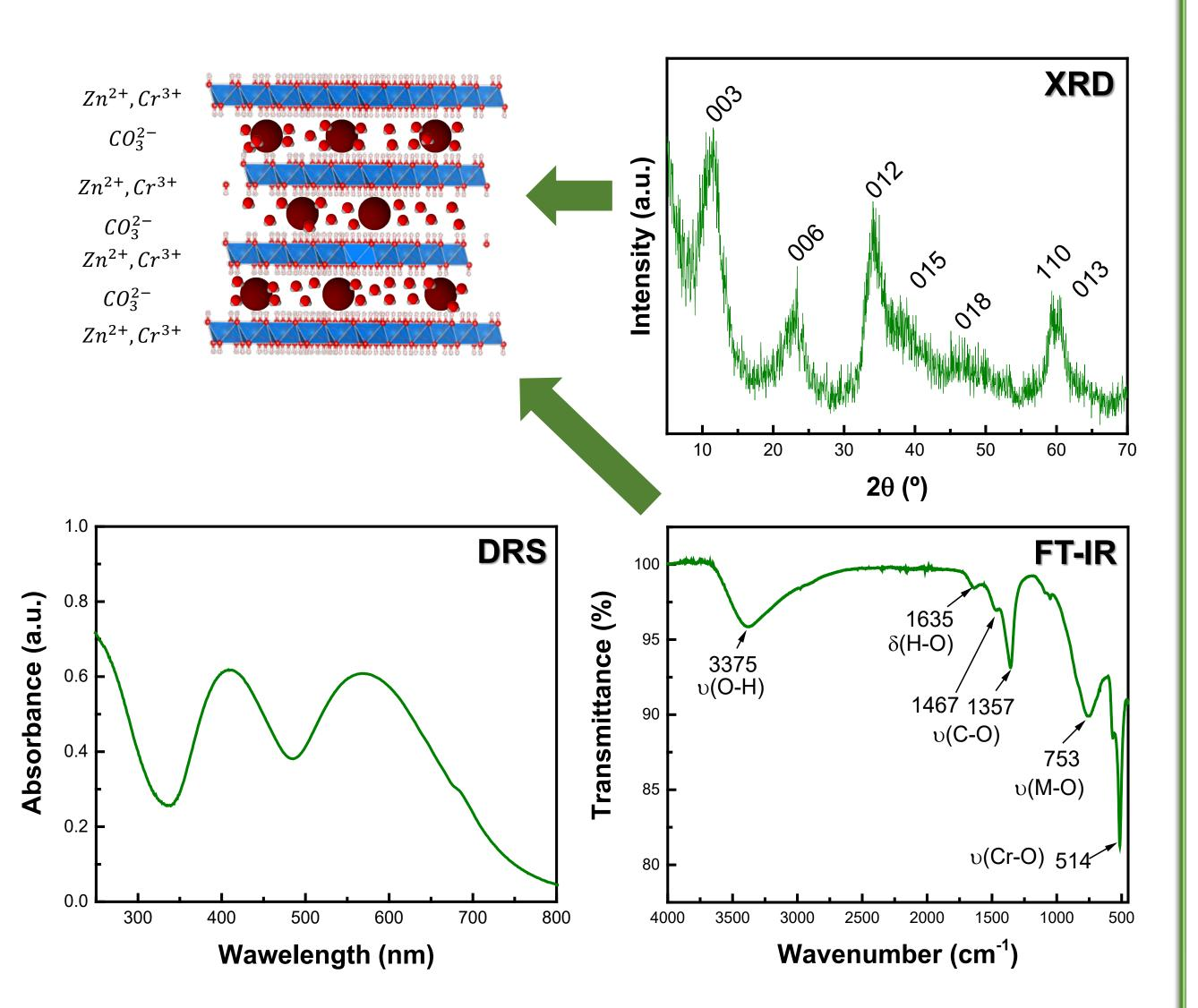
**XRD** pattern characteristic of LDH pure phase with low crystallinity. Characteristic FT-IR spectra of LDH containing carbonate in the interlayer. DRS: ZnCr-LDH can absorb light in a wide range of wavelengths from the UV to the Visible.
